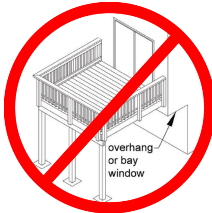
Figure 18. No Attachment to House Overhang
