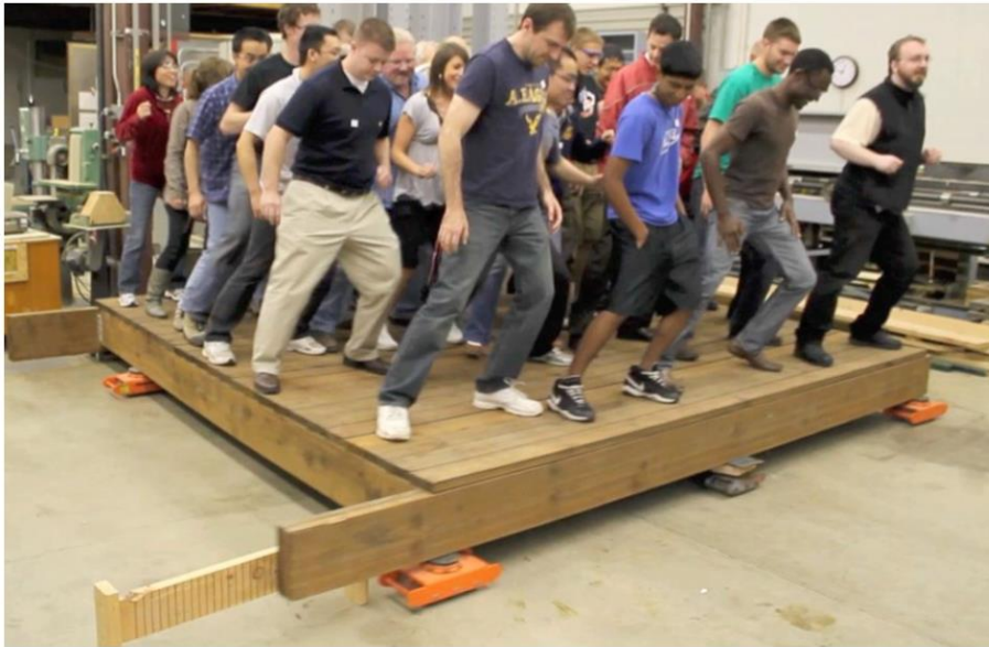
Figure 2. Cyclic Loading Caused by Occupants Swaying Side to Side in Unison
